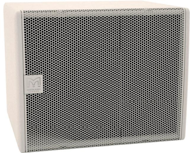
The CSX112 is an ultra-compact direct radiating sub-bass system designed to extend the bandwidth and increase the headroom of CDD full-range models from the CDD5 to the CDD10. It features a very efficient 12" (300mm) long-throw bass driver with a high power 3" (75mm) voice coil and generously-sized reflex ports for low noise, high power operation.
